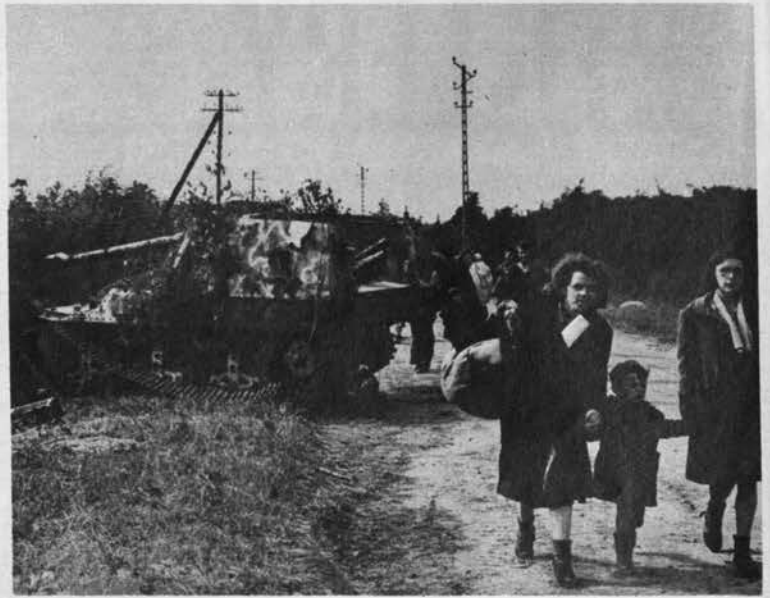
Lorraine tank chassis here mounts a German 75-mm. gun. It has six bogie wheels in pairs with four return rollers and front sprocket.
